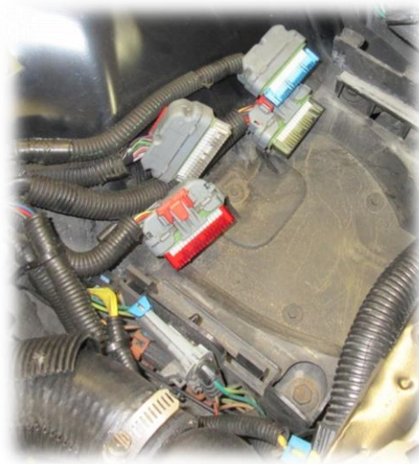
Figure 1 - Stock LT PCM Removed. (B-Body Example)
