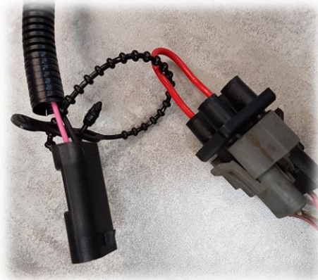
Figure 6 – Black and Gray Ignition Coil connectors connected to coil jumper connector
